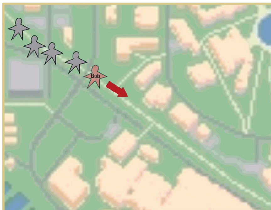
Figure 5. Topiary's cruise control. The tool can automatically update an entity's location on the basis of its current velocity. Wizards can deactivate the function by manually dragging the target entity. (The "gray star men," shown here to illustrate Bob's path, aren't visible in the actual interface.)
