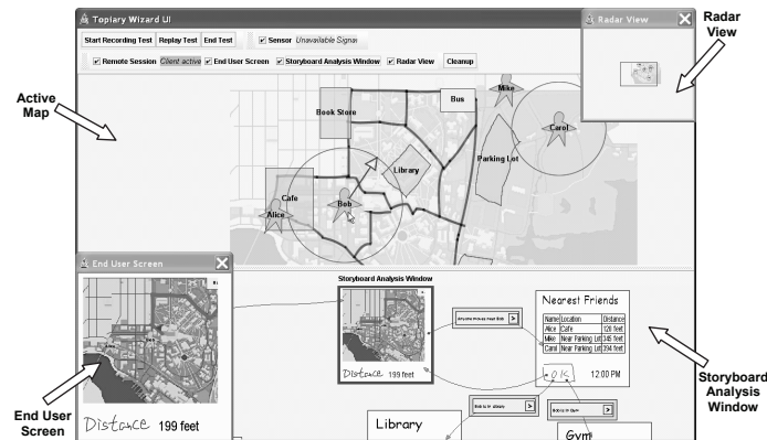
Figure 6. The Wizard UI has four major parts: The Active Map (a clone of the Active Map workspace) for simulating location contexts, the End User Screen for monitoring a user's interaction or debugging a design, the Storyboard Analysis Window for analyzing interaction logic and the Radar View for easy navigation of the Activity Map.
