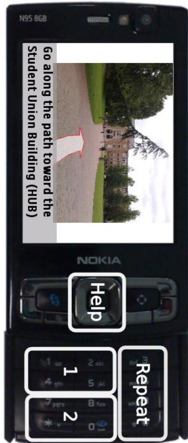
Figure 2. N95 8GB phone used in our study. The keypad was divided into four input areas to request help (alternate direction), repeat directions, and switch between a photo-based direction involving a turn and a view from the turn facing the correct orientation (to disambiguate turn location).
