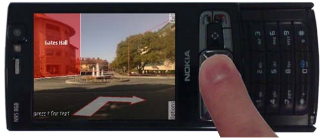
Figure 1: Light-weight mobile client that can display navigational instructions as well as additional context by labelling landmarks and allowing them to be hyperlinked.
